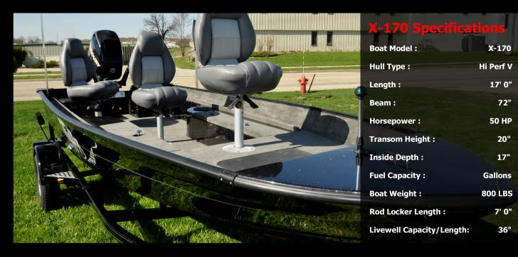
The all new Tuffy X-170 T Esox is the ideal boat for the multi-species angler looking to fish both big and small waters from a fishing-only interior built into a stable, fast, dry riding low profile V hull.
